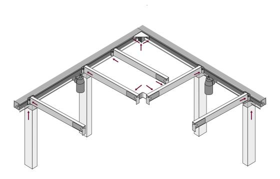
Place the frame against the wall and align it. Adjust the threaded bolts under the legs to ensure that the frame is horizontal.
