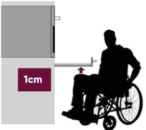
If the client is a wheelchair user, then the underside of the pull out shelf should finish 1cm above the client's knees. The height of the shelf should have been calculated by the designer and added to the plan.
