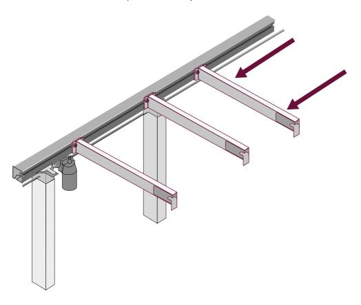
Push the left hand side support arm into the profile. Position it directly above the left leg and fasten it.
