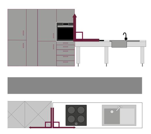
Fit the remaining base units in position around the rise and fall worktop. They should be spaced away from the wall by 60mm to allow for a 650mm deep worktop with the front of the doors flush with the front of the worktop. They should be set out with the same plinth height as the tall units.
