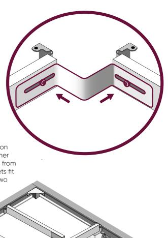
Mount the assembly fitting on the two brackets in the corner of the frame. Move the legs from side to side until the brackets fit as illustrated. Tighten the two screws.
