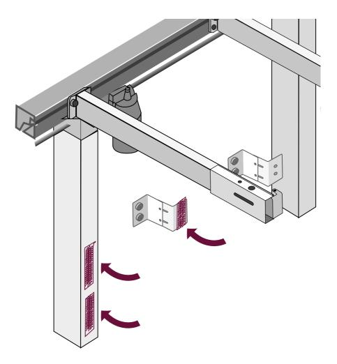
Attach the bottom panel (352mm) to the Velcro. It should be touching the floor, and flush with the units / panels either side.
