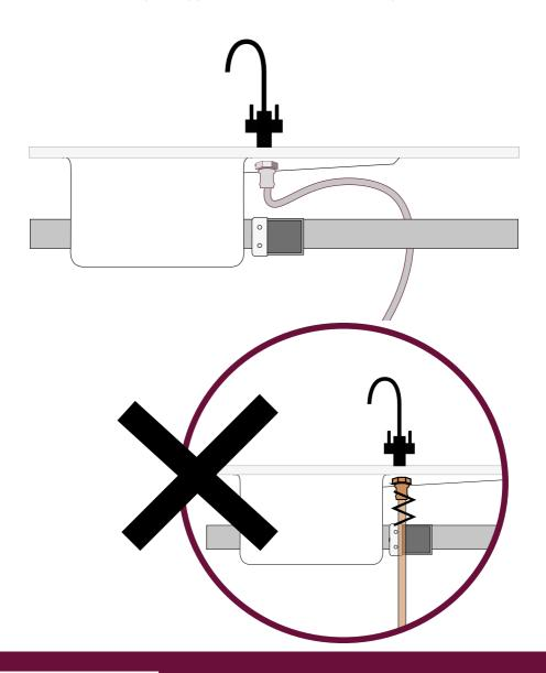
Calculate the location for the hole for sink waste. Drill a 64mm diameter hole, and seal with a suitable sealant.
