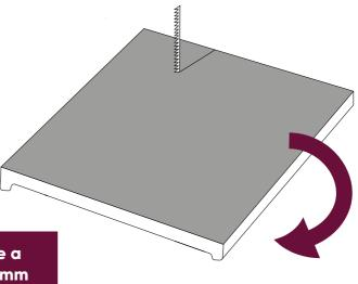
There should be a minimum of 300mm between the sink and hob. Measure this from the appliance edge, not the cut out edge.
