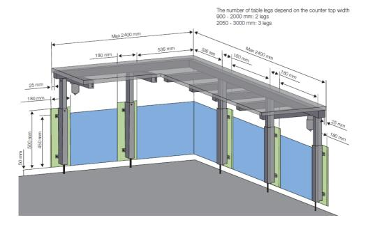
Please note: the frame should not be fixed directly to the wall. Use the distance brackets supplied to space the legs from the wall by 70mm. See page 22 for more detail.
