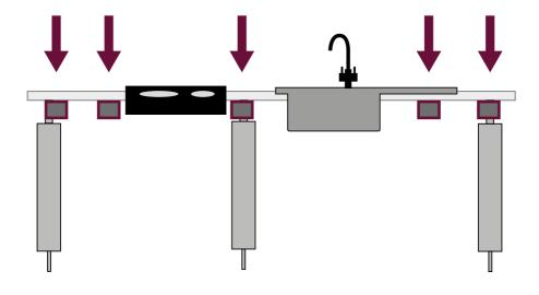
The legs should be positioned so that an arm can sit above each one. Use the calculated positions of the support arms to mark out where to fit the legs on the back wall. Items supplied but not required:
