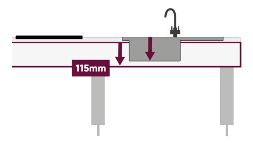
Fascia must be fitted flush with the front/side edge of the worktop. Do not allow any worktop overhang on the rise and fall section, or on the worktop edge next to a rise and fall section.
