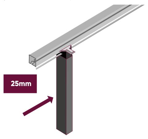
Secure each leg to the aluminium profile with two bolts.
