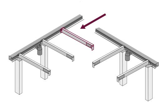
For L shaped rise and fall Slide the two nuts of the angular fitting into the aluminium profile, and tighten the screws lightly.
