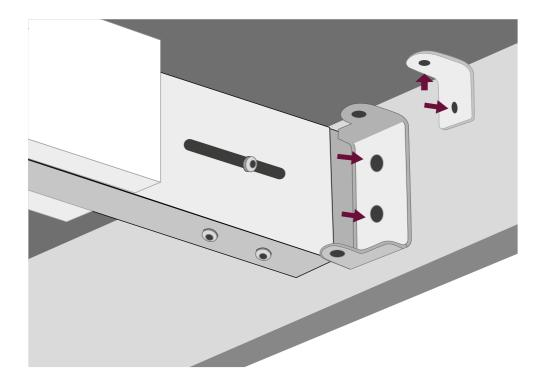
Fascias should be fitted on both sides, and on the back of the worktop if it is open and exposed (e.g. in an island).
