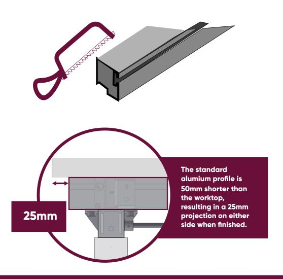
Cut the spindle(s) to the required length (100mm shorter than the aluminium profile) using a chopsaw with an aluminium blade. Soften the sharp edges of the cut end of the spindle with a file.
