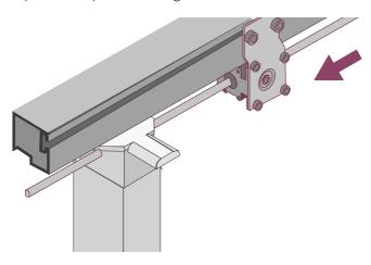
Push the middle support arm(s) into the aluminium profile from the right hand side to the required position and fasten with two screws on each support.
