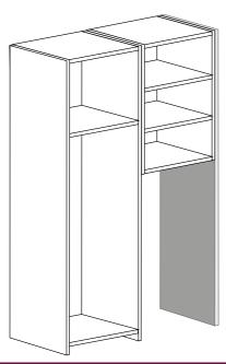
Determine and measure position of open display unit on tall unit. Drill holes through the tall unit side panel to allow the fixings to be hidden when the unit is in position.
