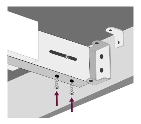
After placing the worktop on the frame you may have to compensate for the weight of the worktop if the frame is no longer horizontal from the wall to the front fascia.
