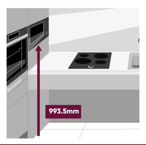
If the design includes a tall unit with a working top door above the adjacent rise and fall, then adapt a tall panel to fit under the working door down to the floor. Use plinth for the 55mm return between the tall panel and the standard plinth under the adjacent tall unit.
