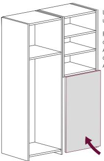
Use spring clips to fix front panel to tall unit and blender panel.
