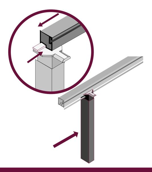
Position the adjustable legs on the aluminium profile. For frames with three legs, place one leg at each end, and one leg in the middle, where the support arms will be positioned.
