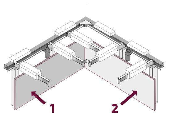
Cut the top panel from 750mm high to 450mm high. Cut the panel in length so that it fits under the worktop with a 5mm gap at each end. Screw the top brackets into the top panel, so that the bottom of the bracket plate is 130mm from the top of the panel.
