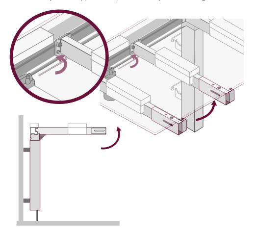
Use a clamp to fasten the front fascia at the required position under the worktop. Press the front fascia fittings forward against the front fascia and fasten with screws from the inside. Use L-Brackets to screw the front fascia to the worktop
