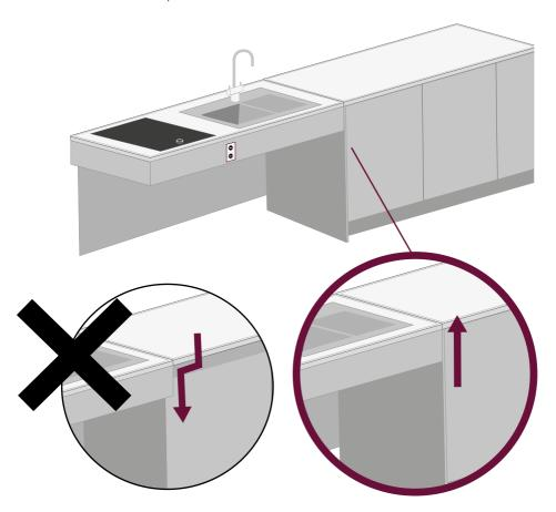
Screw fittings for concealment panel to wall. Adjust them to make sure that the front of the fittings is in line with the front of the legs.
