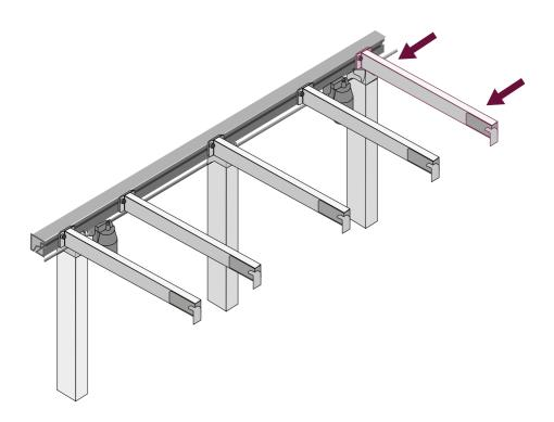
Move the stop rings on the spindle to both sides, so that the stop ring always faces the leg. Secure it by fastening the screw in the stop rings.
