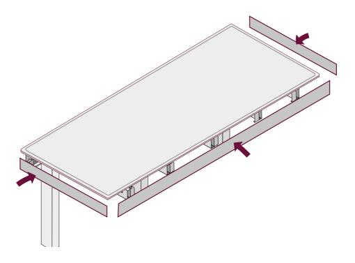
Fascia panel must extend as far down as the sink bowl. The bottom of the sink bowl must not be lower than the bottom edge of the fascia panel. In most cases, 115mm will be sufficient.
