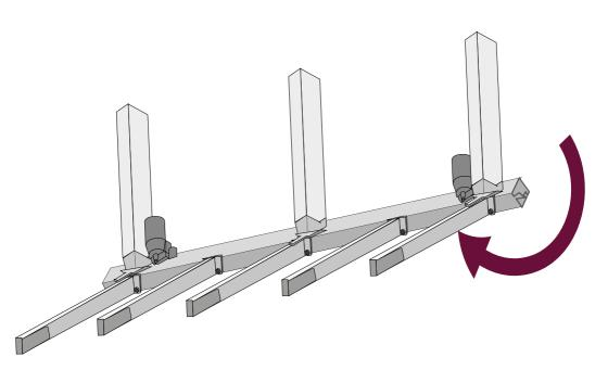
Push the left leg into the groove of the lower side of the aluminium profile.
