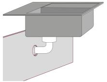
Calculate the location for the hole for sink waste. Drill a 64mm diameter hole, and seal with a suitable sealant. The sink waste does not need to be slotted.
