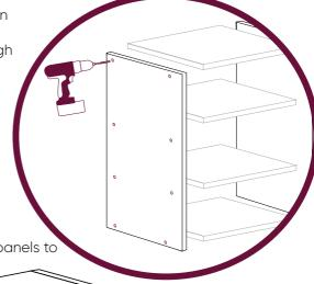
Screw fix top, bottom and mid panels to side panels.
