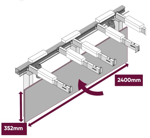
On L shape, fit panels behind hob area first, and panels behind sink area second, to aid removal in case of a plumbing issue.
