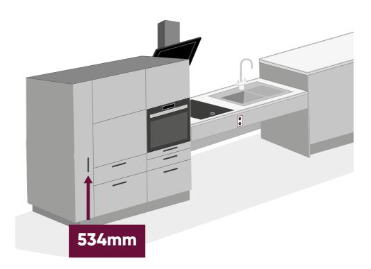
Tile / glass splashbacks can be fitted AFTER the rest of the kitchen. Move the rise and fall to the lowest point and then fit tiles or splashback. Fit the tiles or splashback so that the bottom edge is below the lowest height of the worktop, so that there is no risk of trapping items in the gap between.
