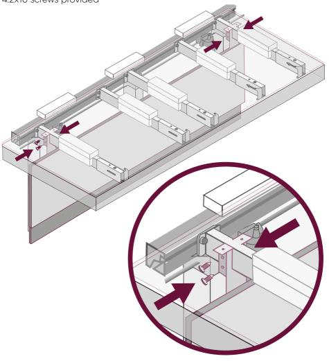
Position the panels so that there is a 5mm space between the front of the bottom panel and the back of the top panel.
