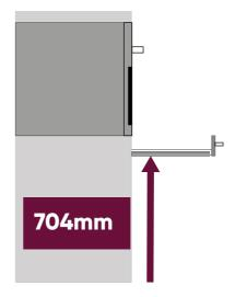
Position the tall bank of units at the appropriate plinth height, with a **60mm** gap between the back of the units and the wall. The 60mm gap allows for the tall blanking panel to sit flush with the frontals, while maintaining an overall depth of 650mm on the tall bank of units.
