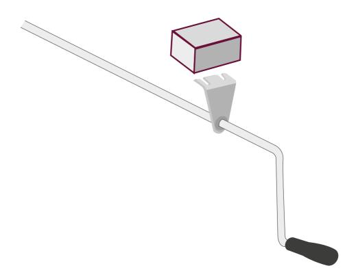
Place the front fascia fittings on the side of the support arm and fasten them loosely by means of the screw provided.
