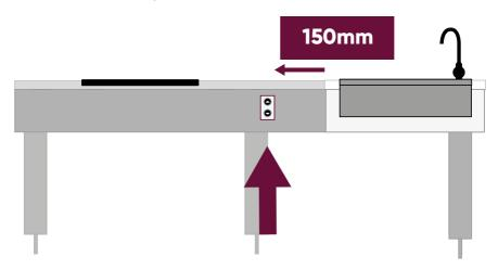
Drill an 18mm diameter hole in the front fascia. Push the cable through the hole in the front fascia from the front. Remove the protective paper on the double-sided tape on the back of the switch, and fix to the front of the fascia.
